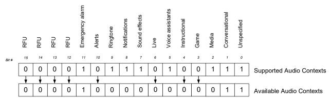
If a bit in the Supported Audio Contexts characteristic is set to 0, the corresponding availability bit (as marked by arrows) cannot change to 1.
