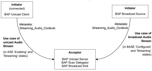
Figure 2.3: Flow of Context Type information as used to signal use cases of unicast and broadcast Audio Streams
