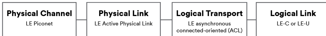
Figure 7.10: Relationship between Logical Link (LE-C or LE-U), Logical Transport (ACL), Physical Link, and Physical Channel
