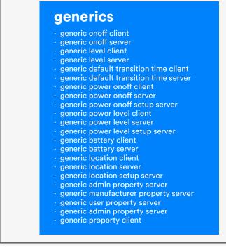
Figure 3 - The Bluetooth Mesh Models
