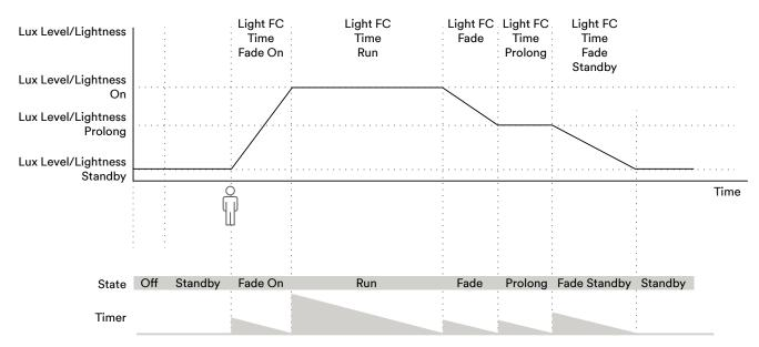
Figure 15 -Lighting controller state transitions
