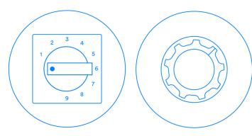
Figure 4a (left) - A 9 x Position Rotary Switch Figure 4b (right) - Analogue Rotary Control
