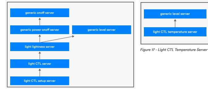
Figure 16 - Light CTL Server and Associated Models
