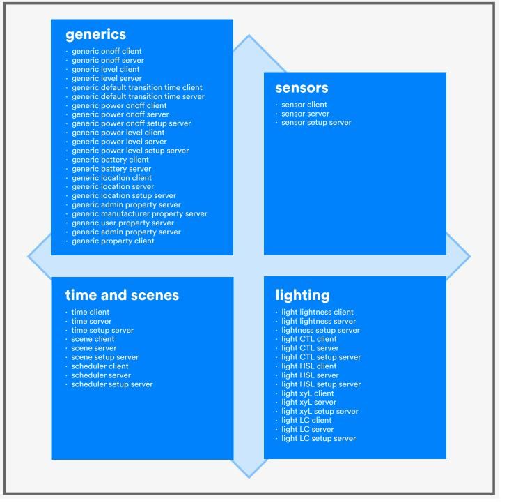
Figure 2 - The Bluetooth Mesh Models
