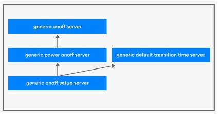
It may not be obvious why the generic default transition time server is part of this picture. The generic on powerup state can be used to define what action to take when powering up, if a transition had been in progress when powering down. Therefore, since this behavior is not triggered by the receipt of a message, which could contain the transition time field, the generic default transition
