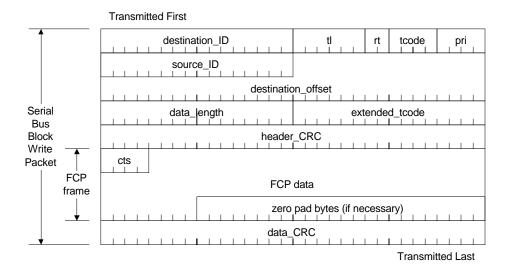
Figure 6.1 – FCP frame within a Serial Bus block write packet
