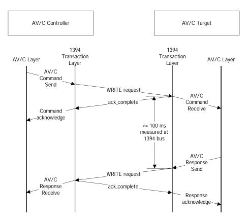
Figure 8.4 – Anatomy of an AV/C transaction with 1394 unified transactions
