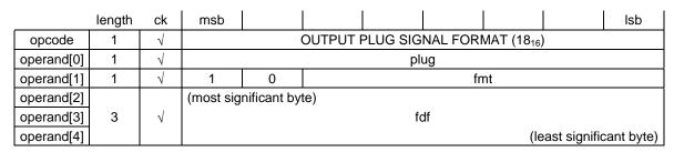
Figure 12.24 - OUTPUT PLUG SIGNAL FORMAT control command frame
