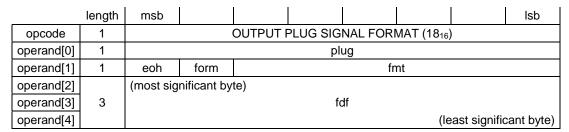
Figure 12.23 - OUTPUT PLUG SIGNAL FORMAT command frame
