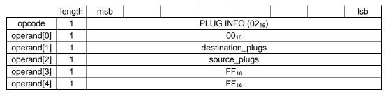
Figure 12.2 – PLUG INFO status command response format from an AV/C subunit
